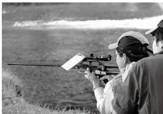
図8. DAN-INJECT社製の炭酸ガス圧式麻醉銃 (CO 2 Injection Rifle Model J.M.ST).
